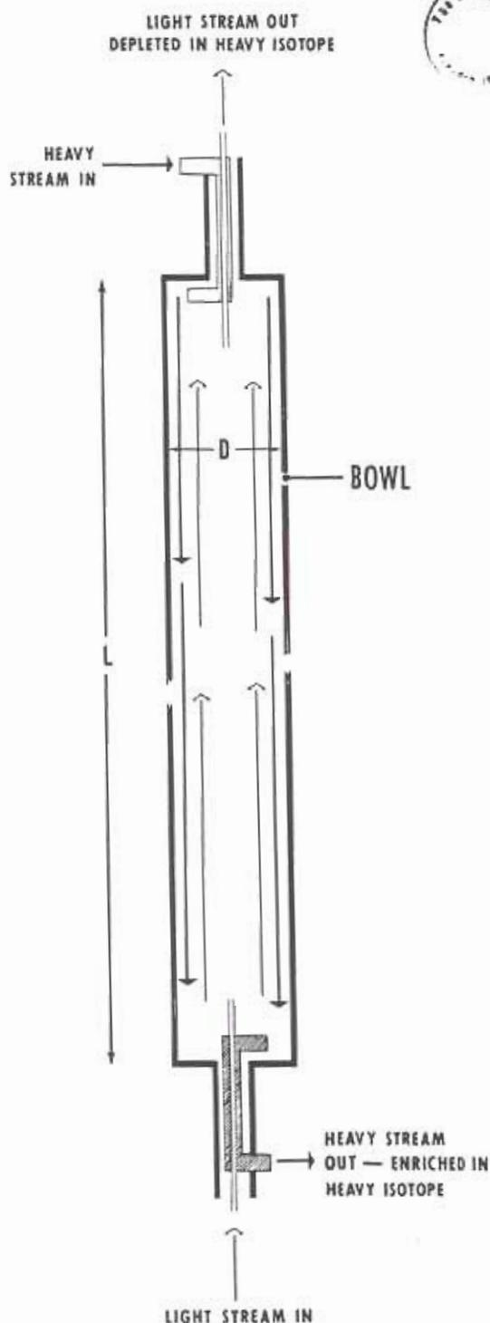
Fig. 1—Schematic drawing of gas centrifuge unit.
